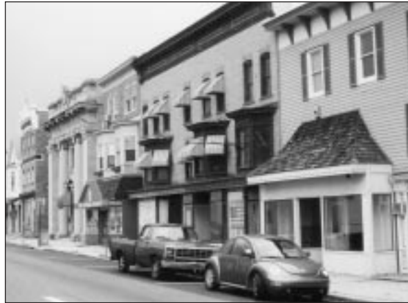
A variety of exterior materials are found in the Market Towns. Frame buildings, such as the one at the right, are now covered with synthetic siding. However, brick and stone buildings predominate the streetscapes.
